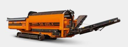
SM 620.2 K Screening area 30.2 m<sup>2</sup> Hopper capacity 7 m<sup>3</sup> Weight 24,000 kg
